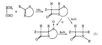
In the synthesis of penams the yield of  $\beta$ -lactams was low when X = H in the thiazoline (4);<sup>7,14</sup> the yield increased sharply when  $X = aryl \text{ or ester.}^{5,15}$  In general, cephams were formed in higher yield than the corresponding penams.
