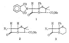
cephalosporins<sup>9</sup> and 4-mercapto-2-azetidinones<sup>10,11</sup> have been synthesized using the "acid chloride method."
